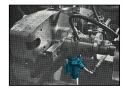
A VT-750-C1 Vacuum Transducer and Cap Unit was selected instead of a Vacuum Sleeve in order to accommodate any number of different dies. Otherwise, individual Vacuum Sleeves would have to be installed in each die. The "A" dimension of .750 insure sufficient clearance for all slugs.
